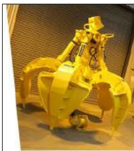
Figure 13: Example grab attached at the end of the crane.
