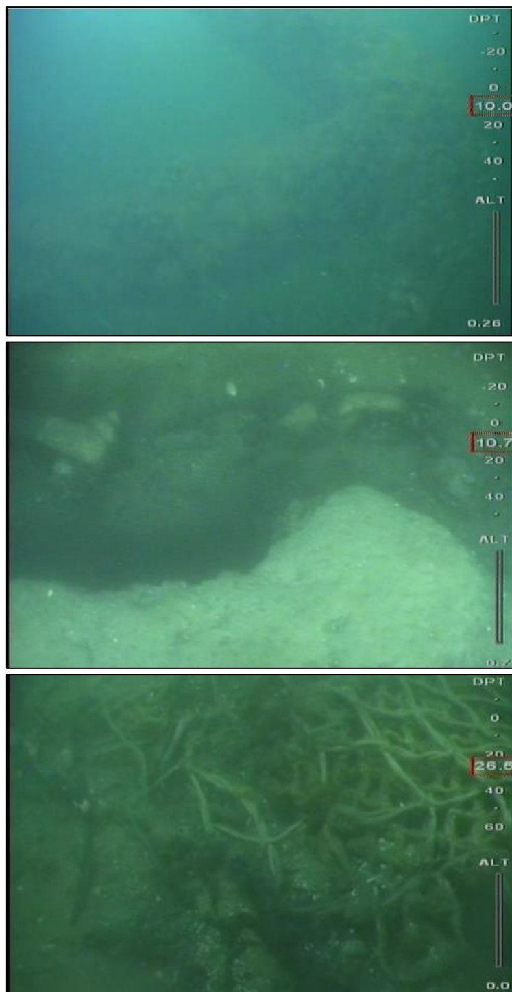
Figure 12: Example of debris identified using WROV, anchor, anchor chain and fishing net (top to bottom).
